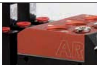
Roscas auxiliares de vacío Vacuum auxiliary ports
